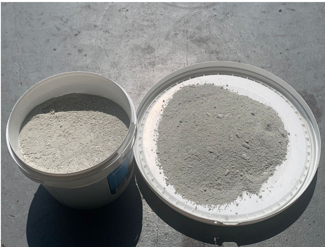
Figure 3: Sample of metal sulfate powder produced from bath pilot batch reactor
