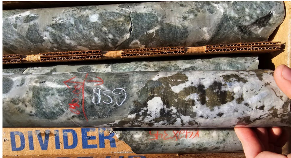
Photo 1 - Sulphides in core in CM23-14
