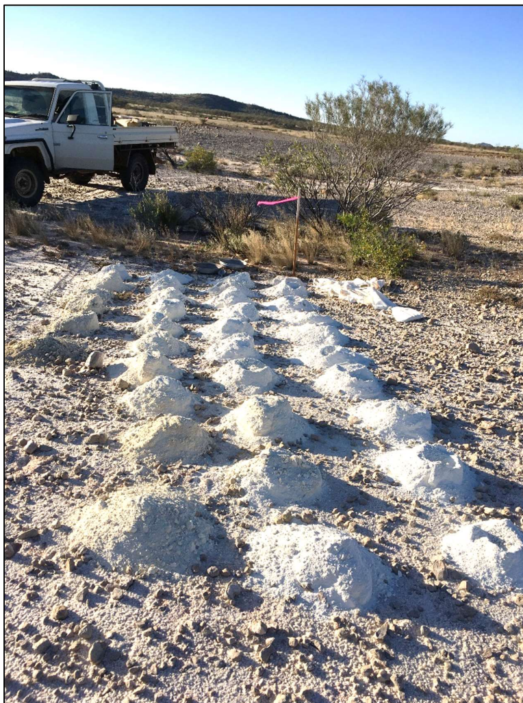
Figure 5 – White, kaolinitic clay-rich regolith materials encountered in hole CCA031 (Crystal Creek prospect).
