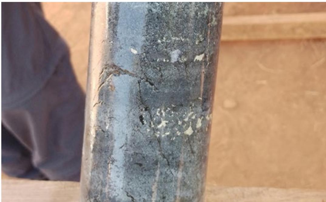
**Figure 3: “Blebby” magmatic sulphides noted within drill hole LPDD004**
