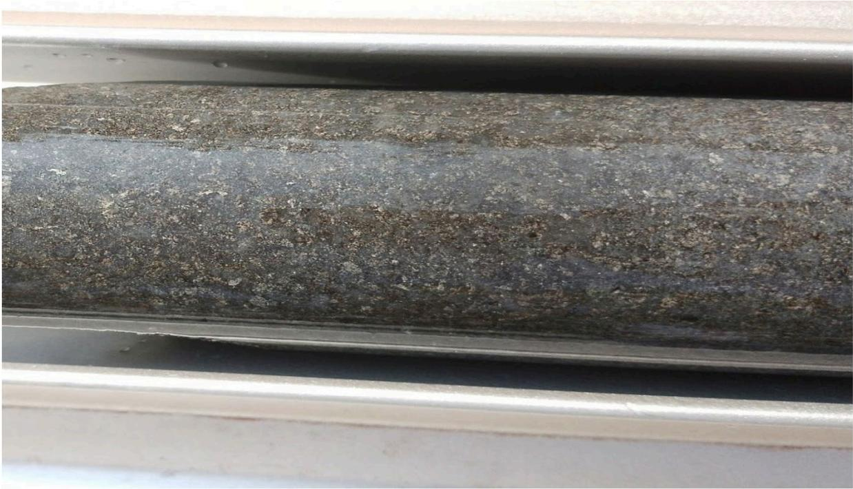
**Figure 2: Initial diamond drillhole core showing mafic rock at Liparamba in which disseminated sulphides have been identified at 40m down hole<sup>2</sup>.**
