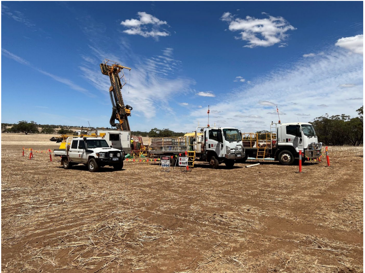
Figure 16: Diamond drill rig at Manning prospect
